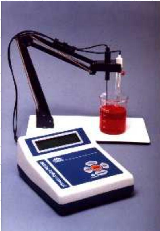
A pH meter can be used to measure acidity.
